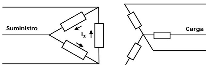
Figure 19 - Delta star isolation transformer
